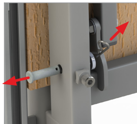
8.1.1 Clevis pin, spacer, and 'R' clip removal
